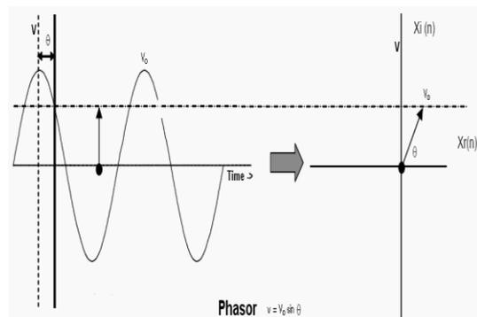
**Figure 1 : Phasor representing magnitude & phase angle of sine wave of voltage or current**
