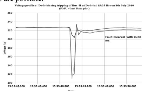
Figure 4 Fault clearing time visualization through PMU
